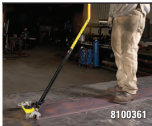
Save time by using on off magnets and wheels to move sheet.
