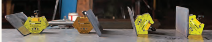
Each Multi Angle offers several common angles: 45/135°, 60/120°, 75/105°, and 90°
