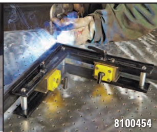
Add MagSquares on each axis for extra holding power.
