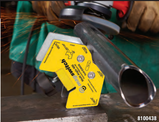
Dual purpose: multi angle workholding tool and quick disconnect and connect vise.
