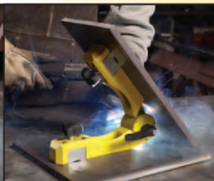
Each magnet holds on two sides.
