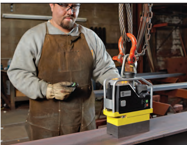
Safety and convenience: one operator remote lifting from a safer distance.
