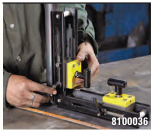
180-degree turn of the knob turns magnet on and off.
