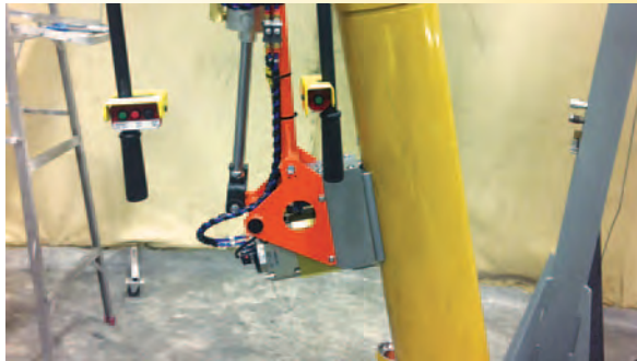
An oil coolant shell and bundle is handled by a PLAY70x2 unit with customized pole shoes. Long and narrow for increased hold on long and round materials with ability to customize poles to match irregular shapes.
