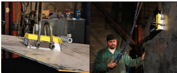
Use the single hook to lift horizontal to vertical.
