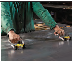
Pivot handle allows use as a hand lifter or a sheet dragger.
