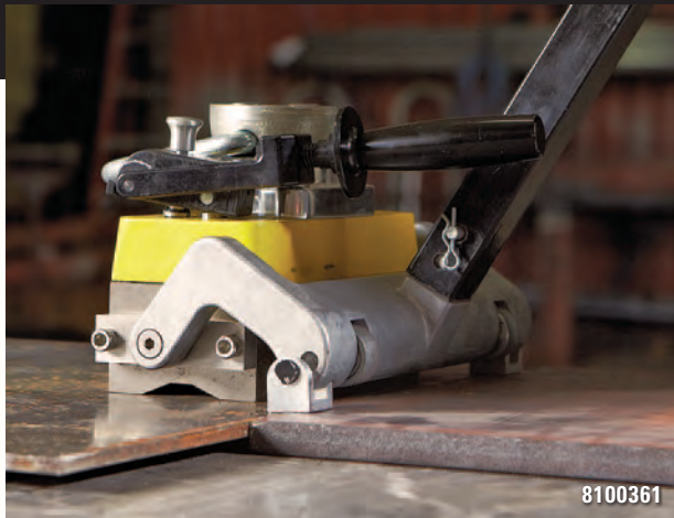
Center Sheet Handler over the seam, turn Magswitch on, press to align and tack.
