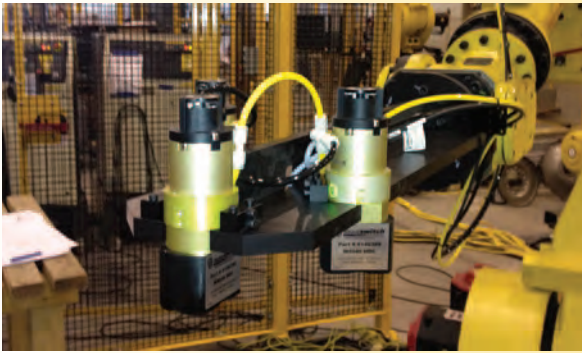
This tool utilizes 3 M4040 magnets to change wheel hub dies in a press. Compact with a powerful deep field to hold strong on flat surfaces.
